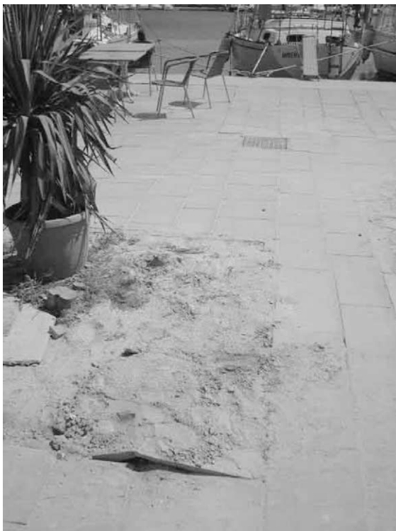
Fig. 16. Sand boil in the seaside in the town of Lefkada, sample ID: LEF1 (photo taken by Papathanassiou, 15/08/2003).
