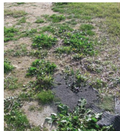
Figure 16. Spots of sea sand that was ejected during soil liquefaction caused along a ground crack opened to the south of Lixouri port with the first strong earthquake.
