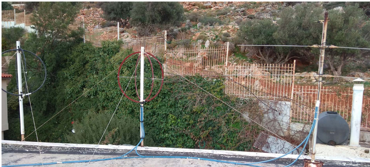
Figure 11. A typical ELSEM-Net remote telemetric station antennas installation at Neapoli, Crete Island (35.2613° N, 25.6103° E), station code “E”. Left mast: the two 10 kHz small loop antennas (black); middle mast: the two 3 kHz small loop antennas (red); right mast (top): the 46 MHz \lambda/2 dipole antenna; right mast (bottom): the 41 MHz \lambda/2 dipole antenna.
