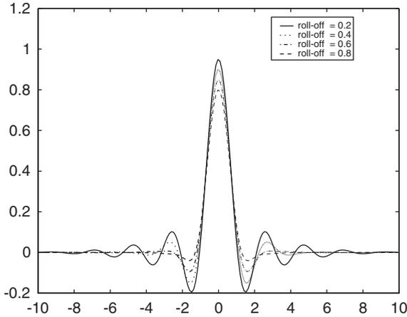
Fig. 4. Raised cosine autocorrelation function for different roll-off factors.
