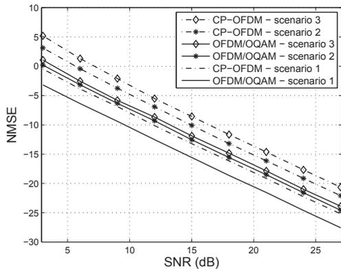
Fig. 2. Estimation performance for channels of low to mild frequency selectivity.  $M = 64$ ,  $K = 3$ .
